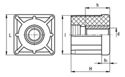
$\begin{array}{ll} d & = M10 \\ h & = 10 \\ H & = 31 \\ h1 & = 6 \\ Internal tube size = 26.0 \\ I & = 26.0 \\ L & = 30 \\ \end{array}$
